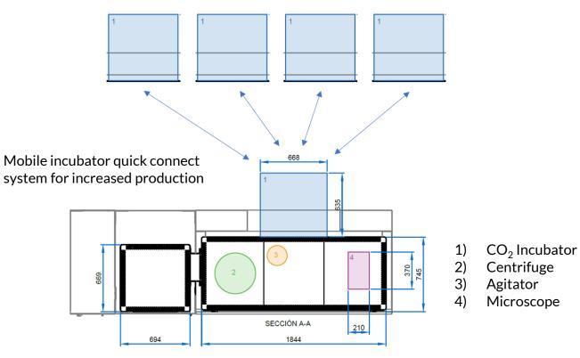
Isolator system for production of Mesenchymal cells
