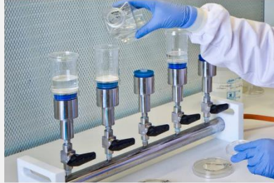
Transport sample to Lab and filter water through Membrane Filter
