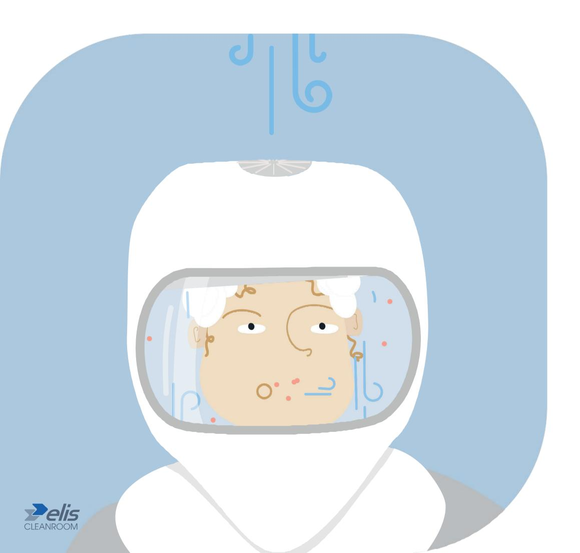
The exhaled CO<sub>2</sub> accumulates and is pushed downward, preventing the operator from inhaling it again. The airflow within the garment is carefully directed through the fabric barrier in a controlled manner. All verified through technical testing.
