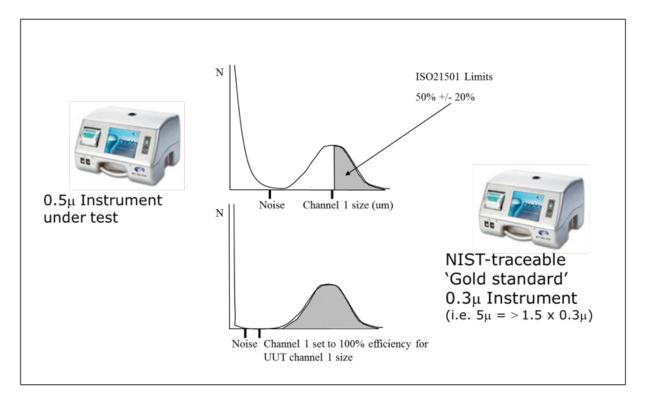
Figure 3. The ISO 21501-4 Counting Efficiency Test
